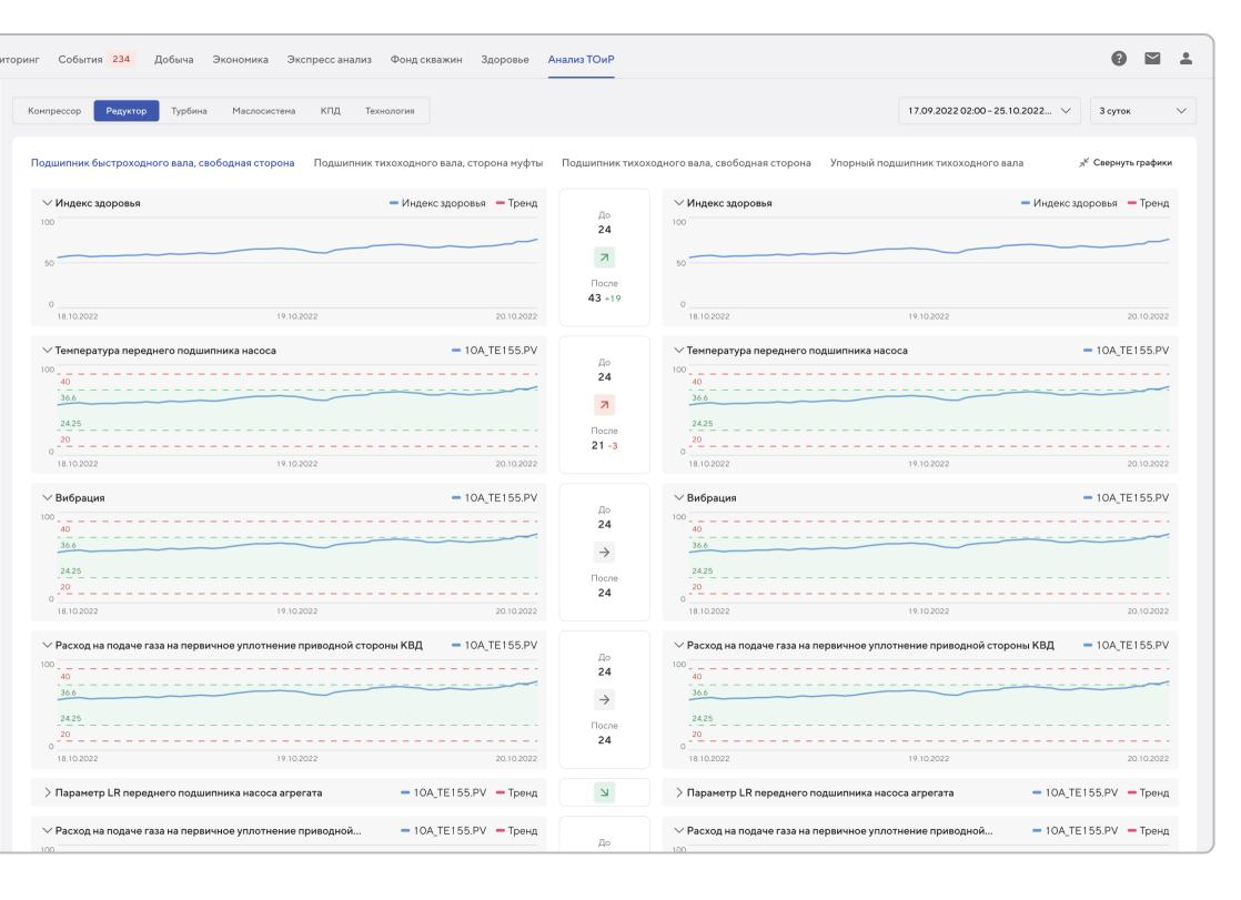
Tailor-made interface to compare equipment condition before and after maintenance
